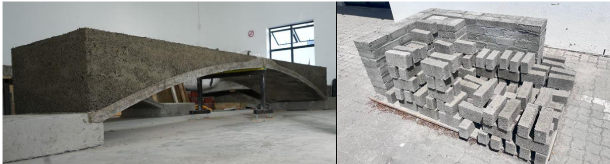
Figure 2. View of a 1 m wide section of completed nonCrete floor and bricks.
